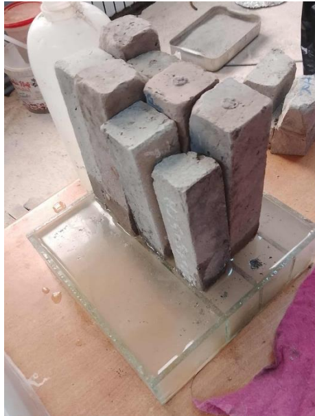
Figure III.15: Essai Absorption capillaire
