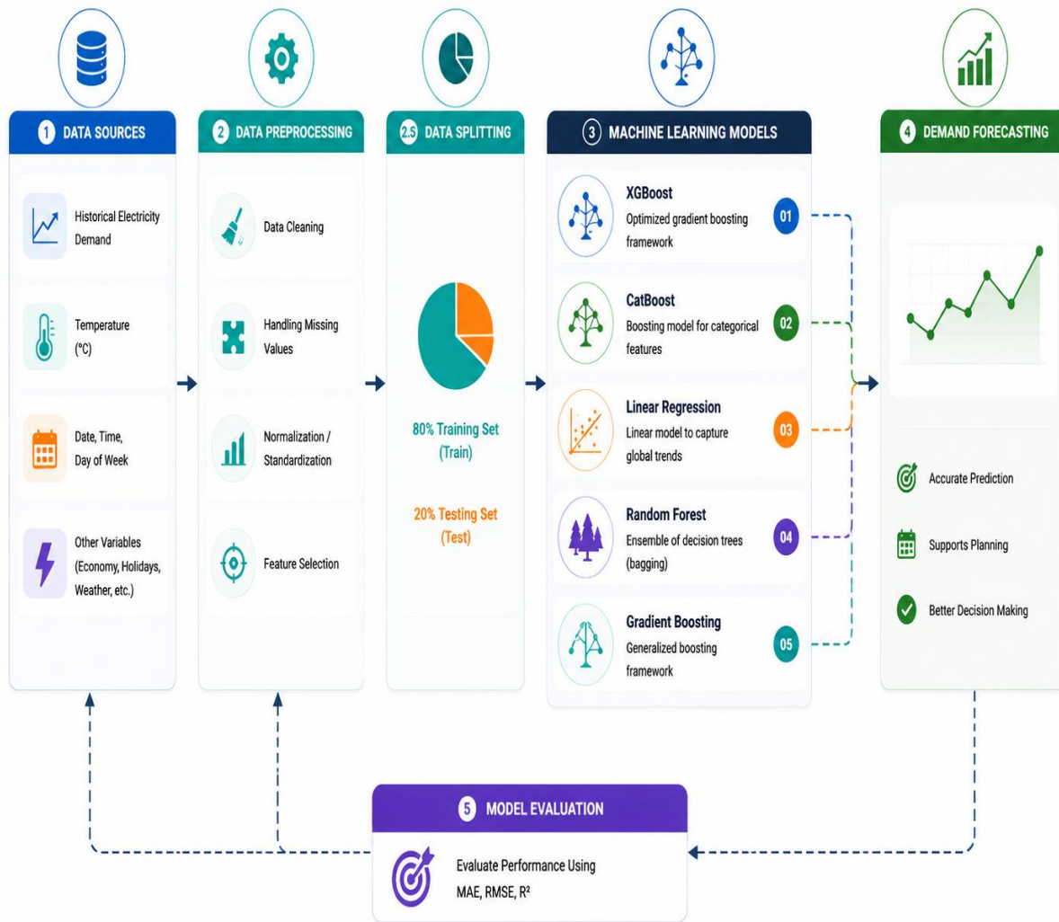
Figure 26: Prediction framework of the proposed photovoltaic forecasting approach.
