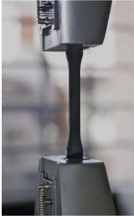
Figure 23: essai de fatigue
