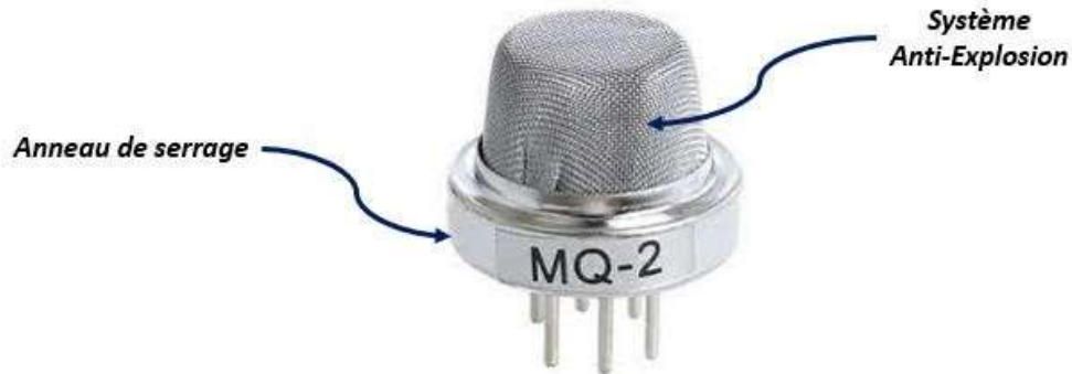
Figure II.7: La structure extérieure de MQ2. [28]
