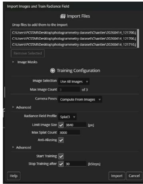
Figure 65: PostShot's image import setup interface and model training. (Ours)
