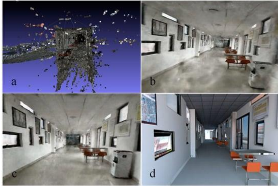
Figure 59: Comparison Chart of Rendering Effects Among Different Algorithms: (a) COLMAP; (b) NeRF (Instant-NGP); (c) 3DGS; (d)Real. (Fang, Zhang, Tan, Liu, & Yang, 2025)
