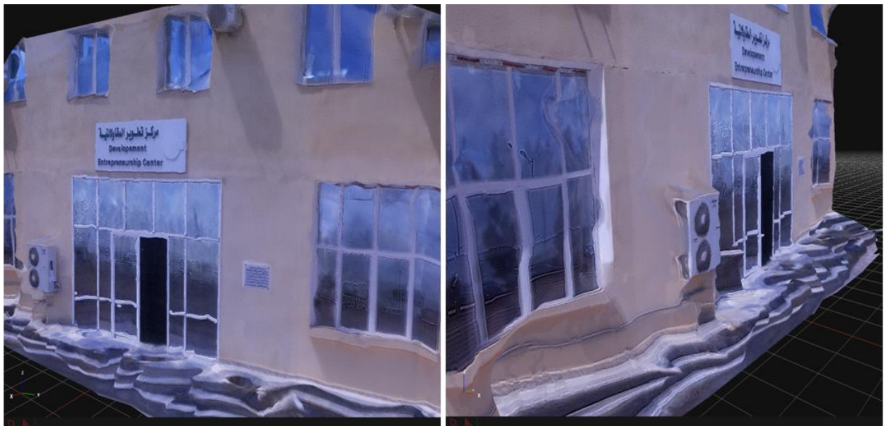
Figure 33: SfM results on a building with highly reflective glass surfaces (Ours)
