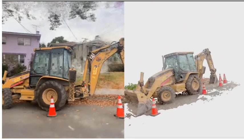
Figure 49: Novel view synthesis of Backhoe Loaders Using Neural Radiance fields (NeRF). (AR-MR-XR, 2022)
