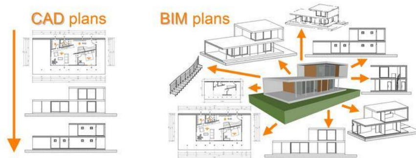
Figure 3: CAD and BIM WORKFLOW COMPARISON (Sharma P. , 2025)
