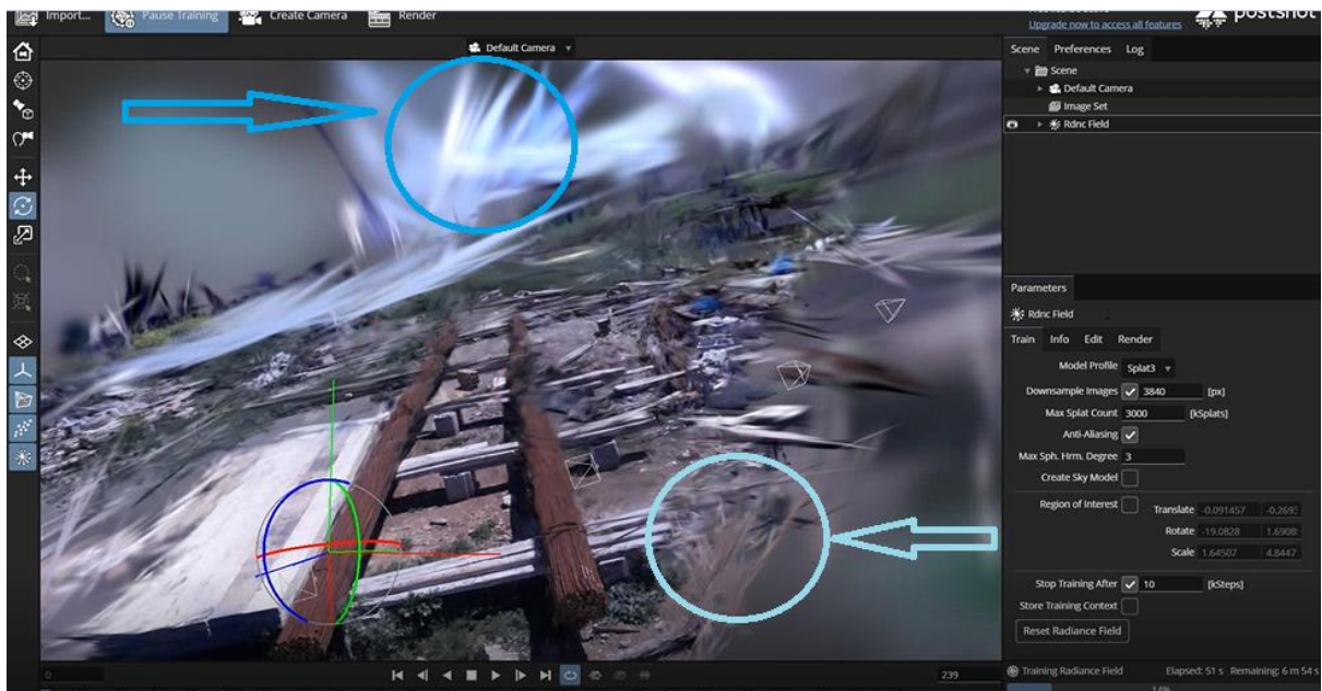
Figure 66: AI training radiance field for Gaussians splatting on Postshot (Ours).
