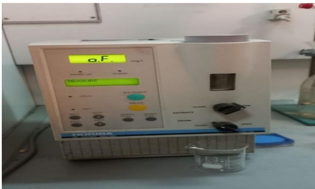
Figure I.7. Analyzer for oil and fat content in water.
