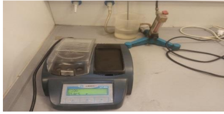
Figure I.8. HACH LANGE LT 200 thermoreactor used for COD analysis.
