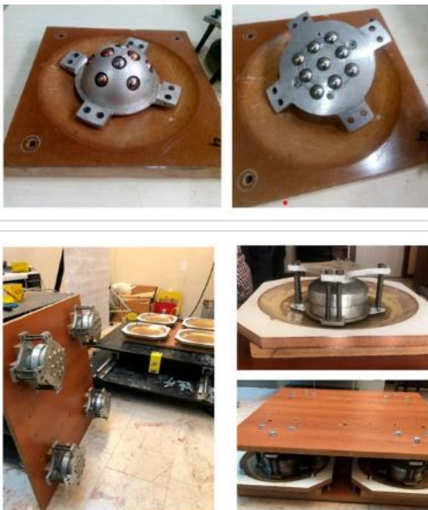
Figure 26 Seismic isolator and components
