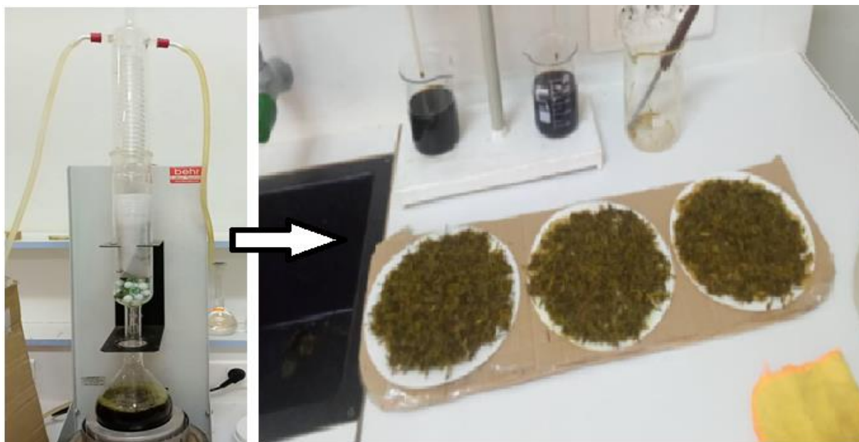
Figure 3 : Solid-liquid extraction of Cellulose by Soxhlet
