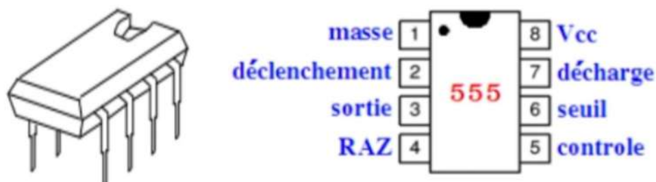
Figure II.10 : Brochage du circuit NE555 [76].
