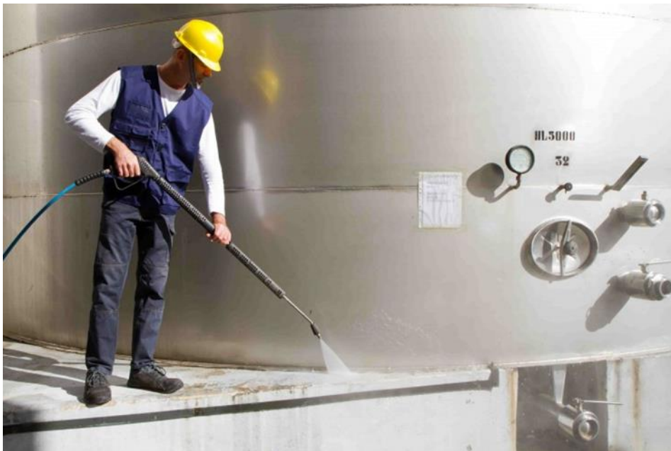
Figure II-8 : nettoyage a pression .
