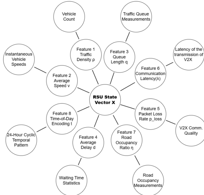
Figure II.5: Composition of the Roadside Unit (RSU) State Vector X.
