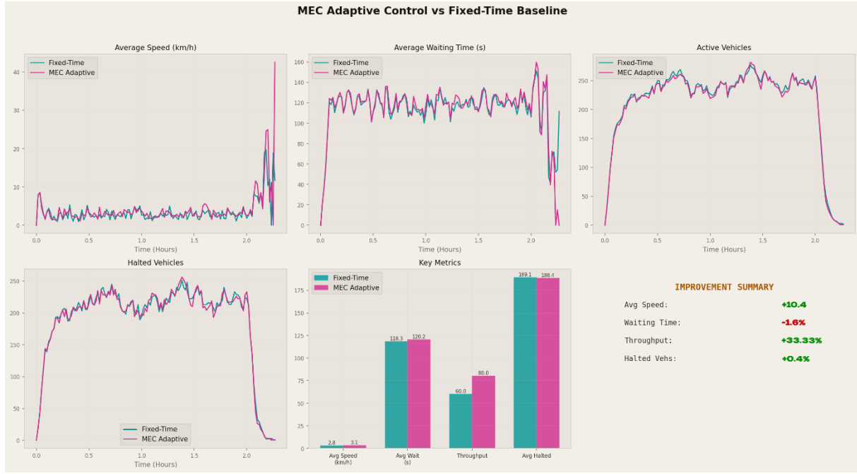
Figure IV.10: MEC Adaptive Control vs Fixed-Time Baseline — full simulation comparison. Top row: Average Speed, Average Waiting Time, Active Vehicles time series. Bottom row: Halted Vehicles time series, Key Metrics bar chart, and Improvement Summary. The +33.3% throughput gain is the primary operational result.
