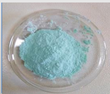
Figure 7: Hydroxyde double lamellaire Nickel-Aluminium
