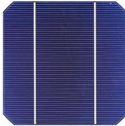
Figure (II.10) : Cellule en silicium monocristallin [42].
