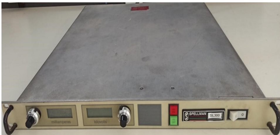
Figure II-2: DC high voltage power supply (SPELLMAN SL300).
