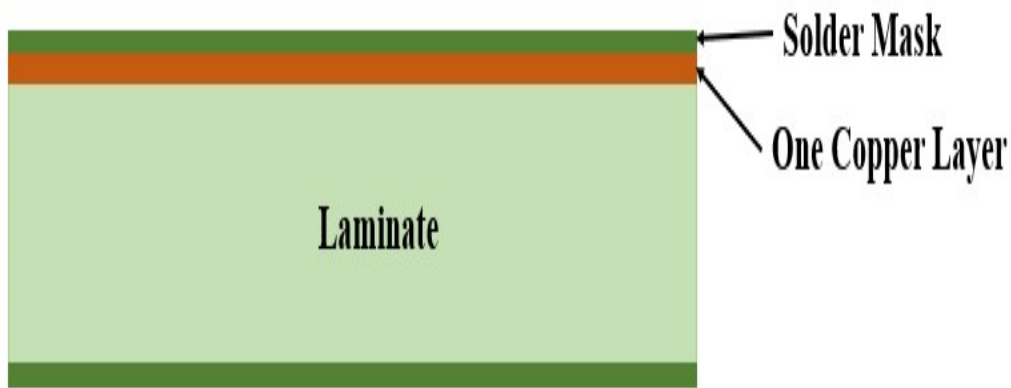
Figure II-17: Single Sided Printed Circuit Board.
