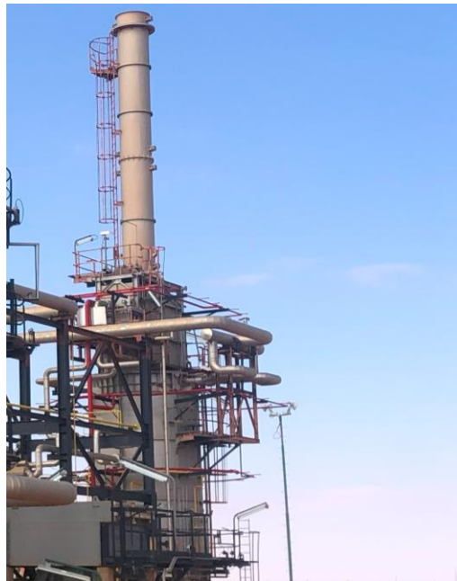
Figure II.6. Industrial Reboiler System for Depropanizer Column.
