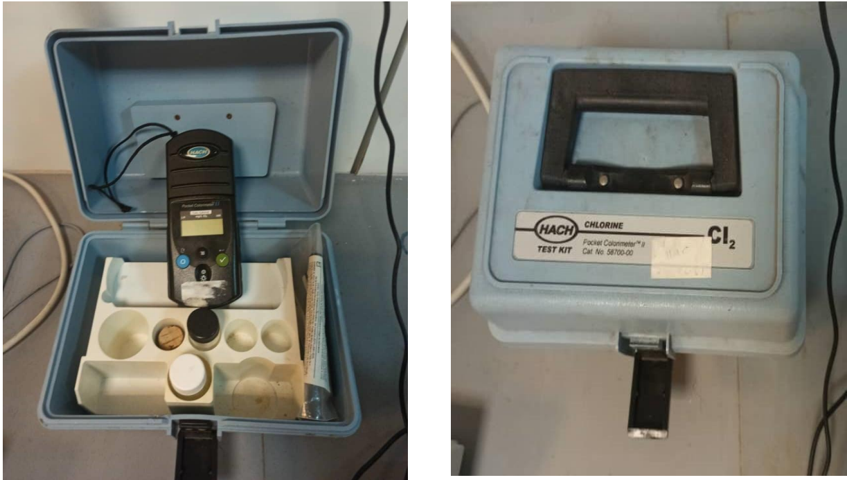
Figure I.5. Hach portable colorimeter for free chlorine.
