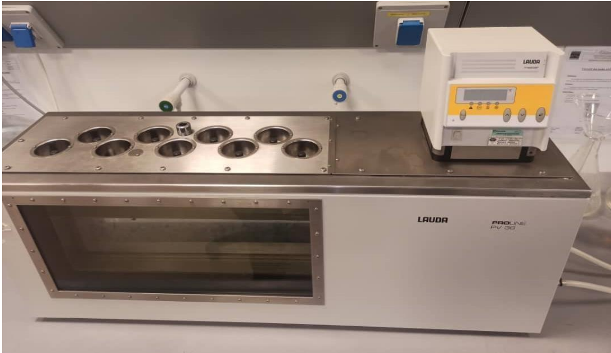
Figure I.6. Lauda proline PV 36: thermostated bath for viscosimetry.
