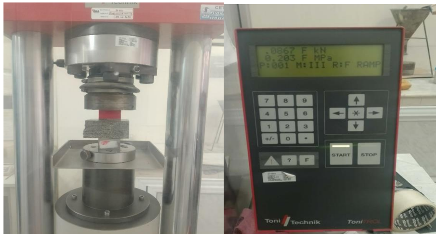
Figure II.38. Essai de Compression
