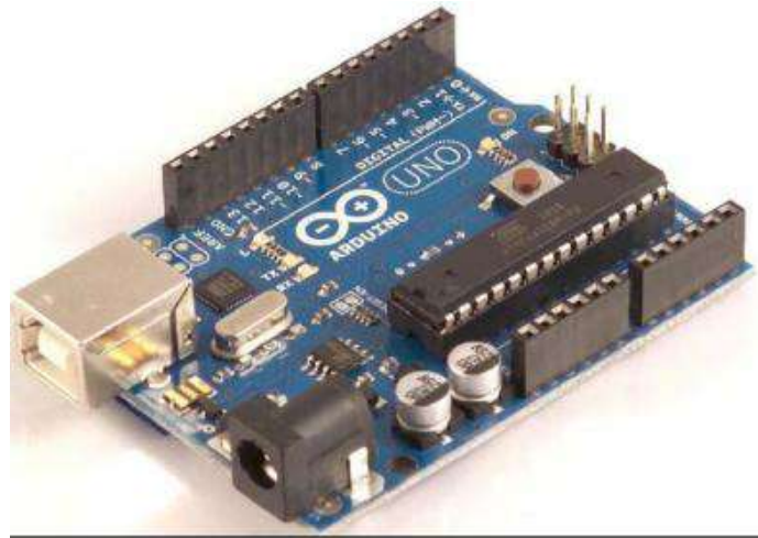
Figure II.9. La carte Arduino UNO.[22]
