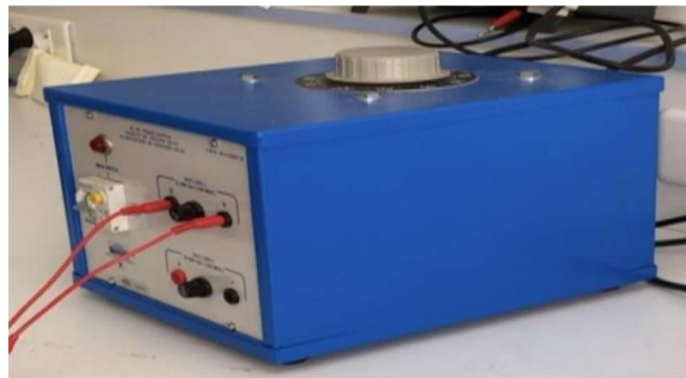
Figure II.8: Photograph of the auto-transformer.
