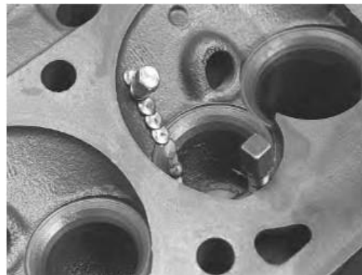
Fig 40: Pinning a crack. Drill both ends of the crack.
