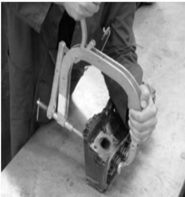
Fig 34: Valve spring compressors. A common type of valve spring compressor in use.
