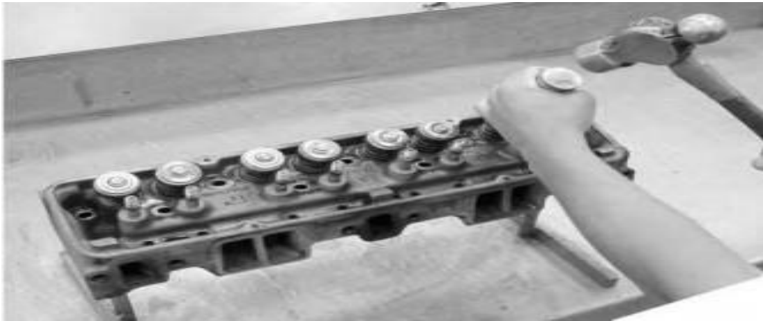
Fig32: Verify that the cam caps are correctly numbered before removing them
