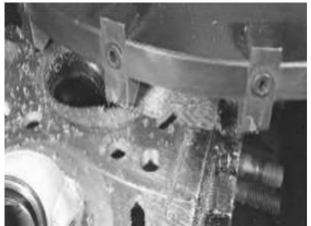
Fig 45: A circular pattern left on the head during machining.
