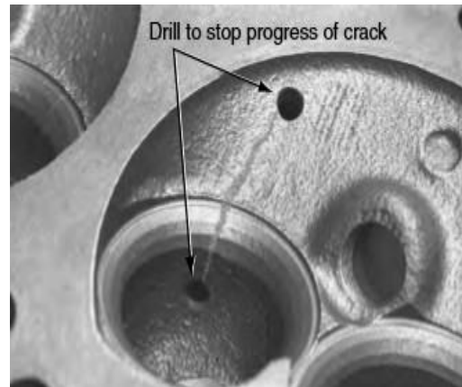
Fig 40: Pinning a crack. Drill both ends of the crack.
