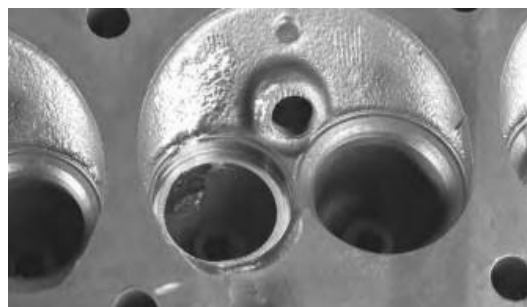
Fig 42: Grind and clean the chamber.
