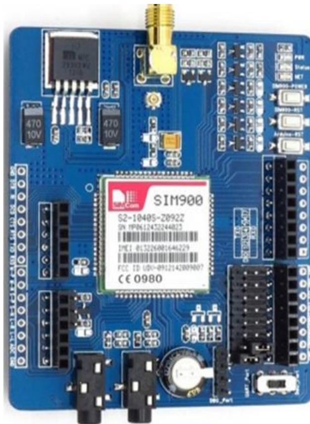
Figure III.10: Module GSM (SIM900). [28]
