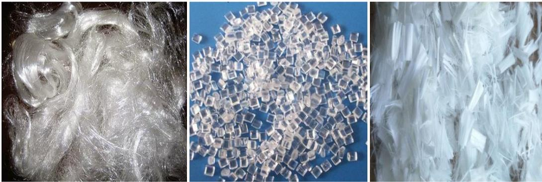
**Figure 3.5: les fibres polyamide, PVC, PP**
