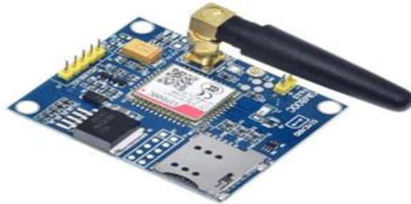
Figure II.2: Module SIM800C. [W6]
