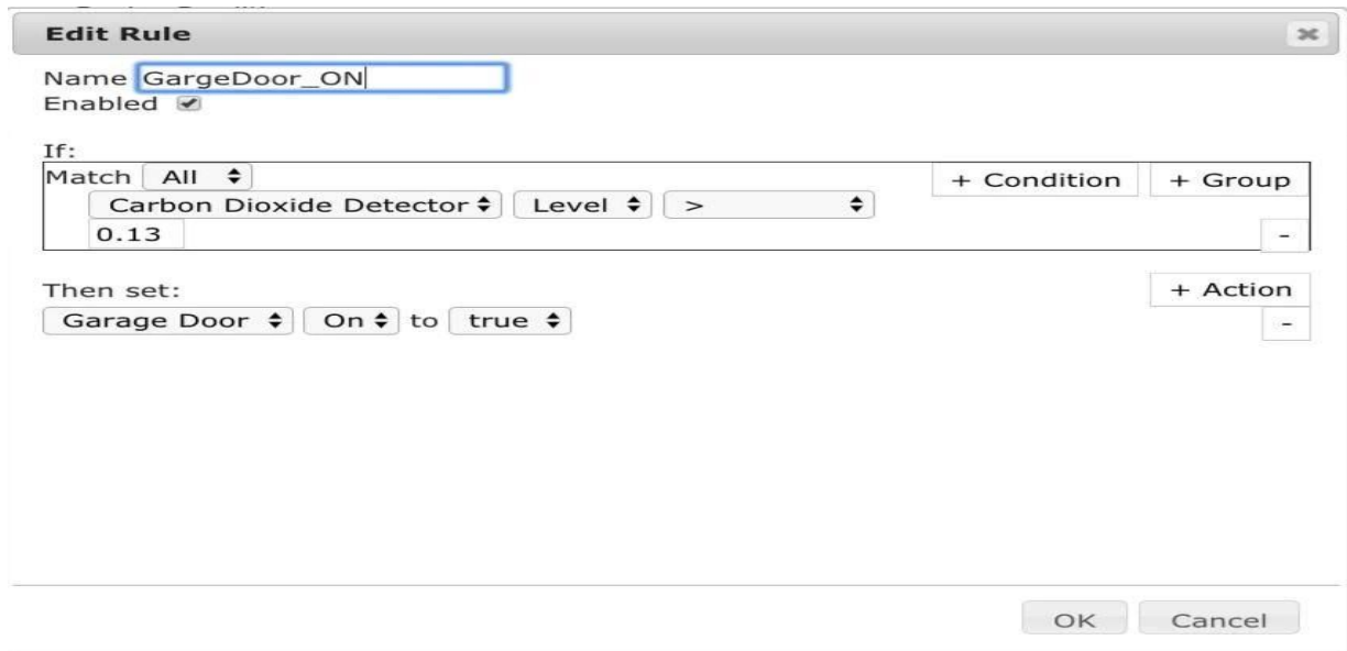
Figure 50: La condition GargeDoor_ON.
