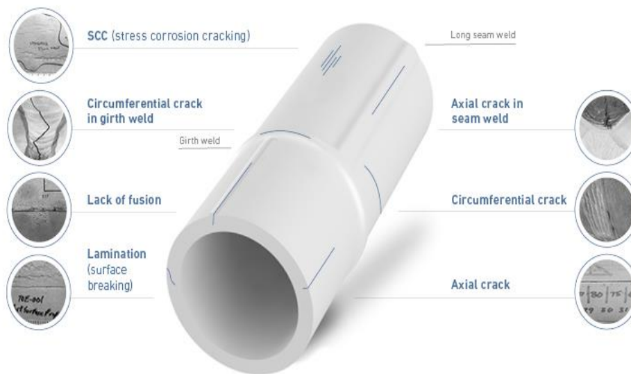
Figure 2- 12 The various types of cracks [40].
