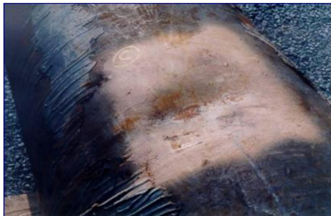
Figure 2- 13 A dent on a pipe [44].
