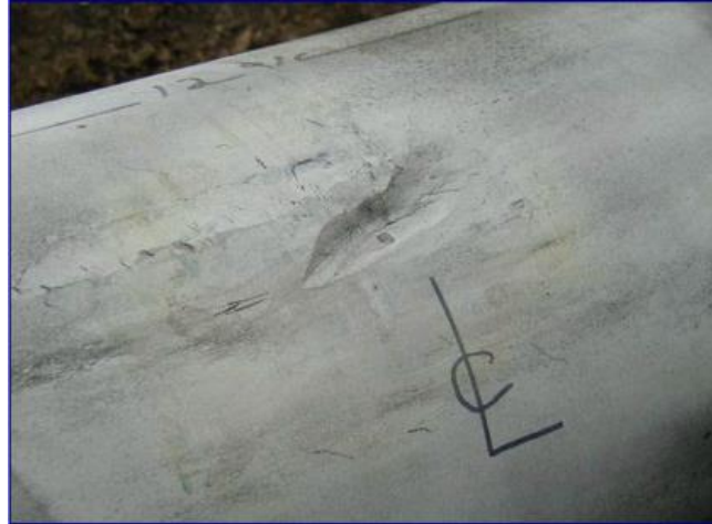
Figure 2- 14 A gouge or a scratch [44].
