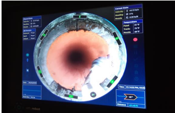
Figure 2- 17 Jettyrobot in an inspection and cleaning process [47].
