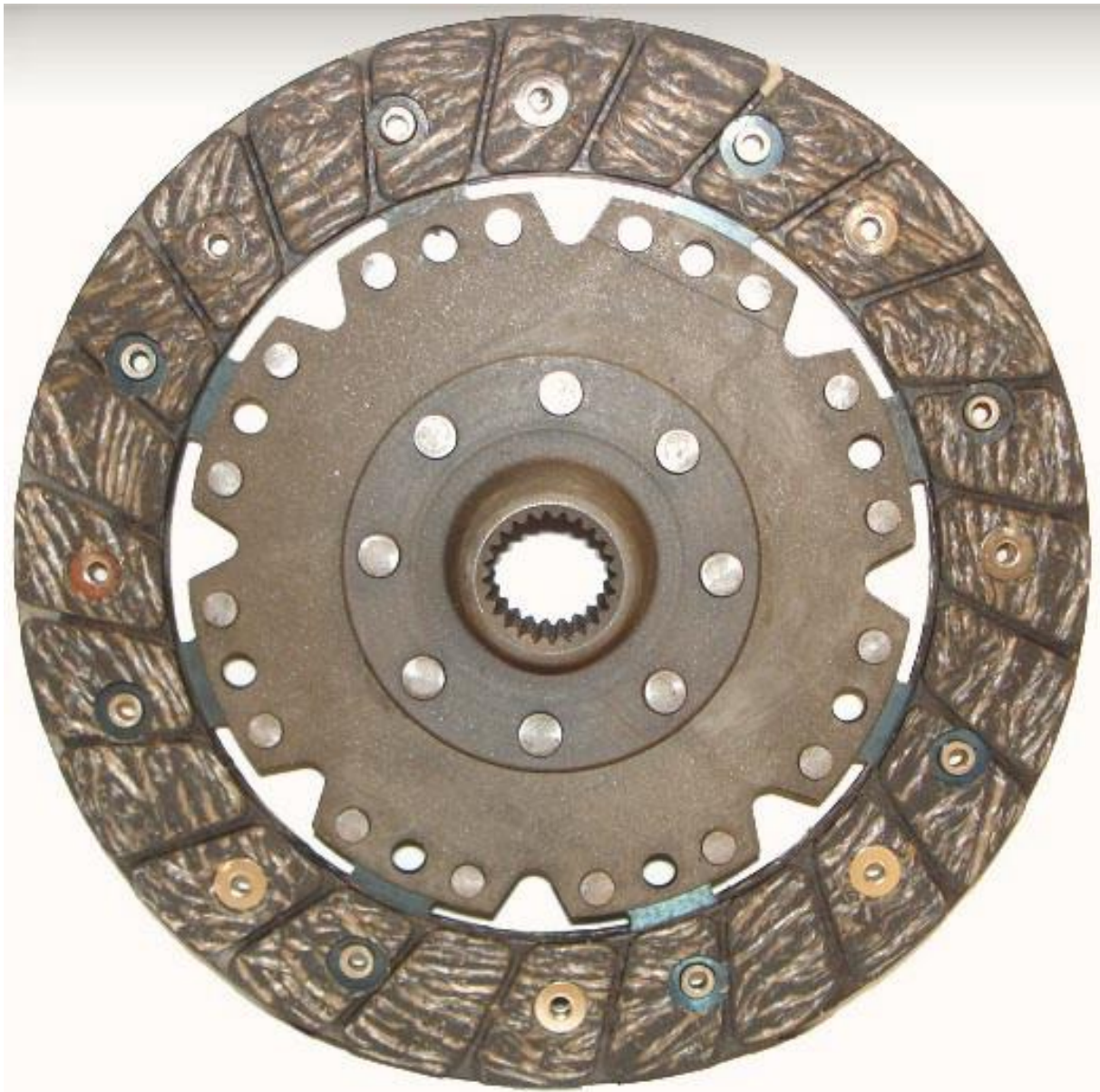
Figure I.21 : Disque sans ressort [21]
