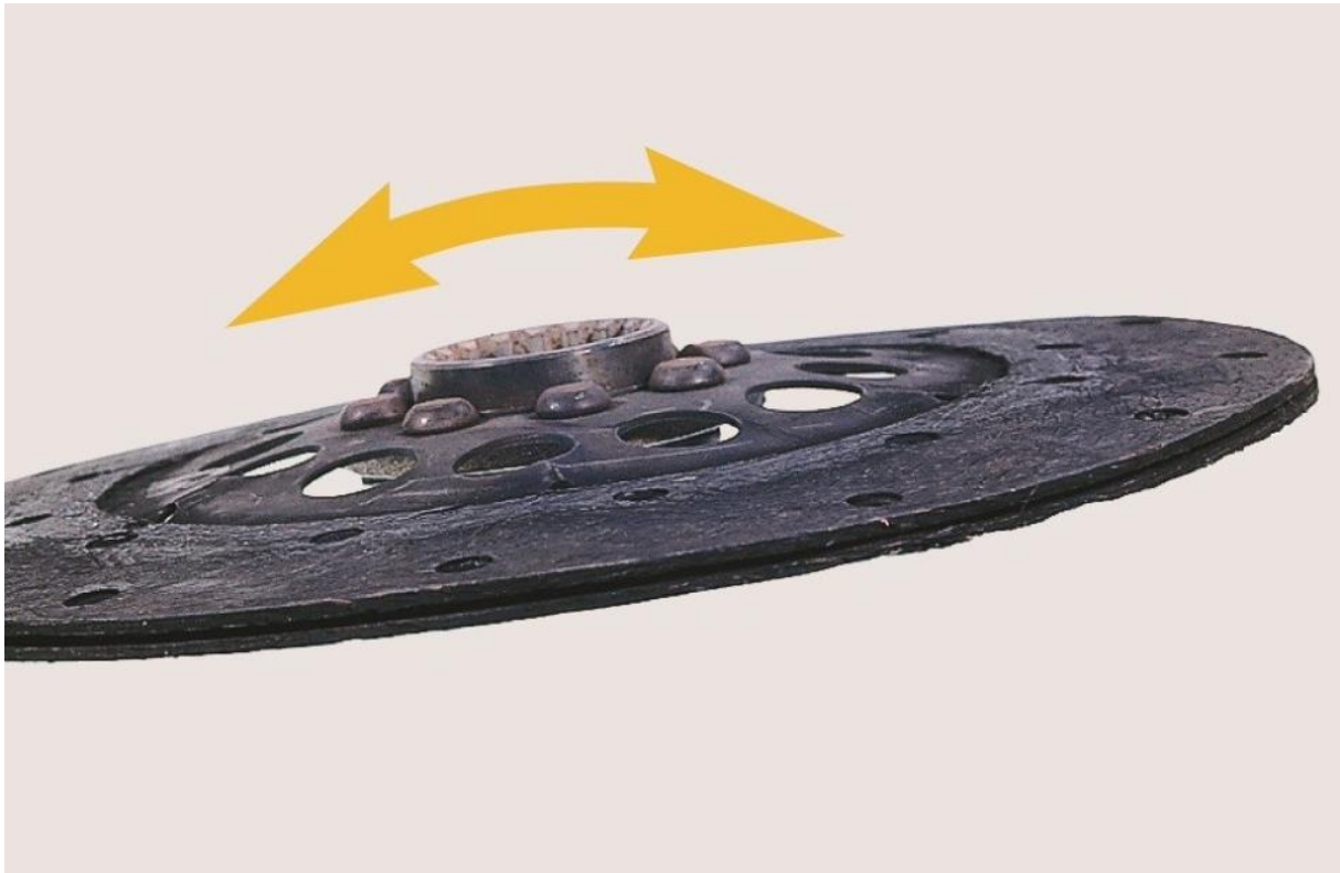
Figure II.4 : Un disque bombé [34]
