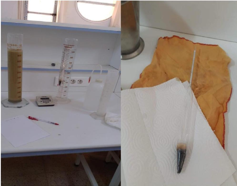
**Figure 31:** Appareillage sédimentation[2]
