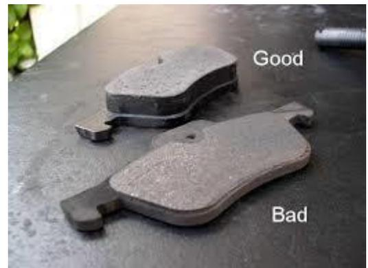
Figure 30: Usure excessive des plaquette(1-31)
