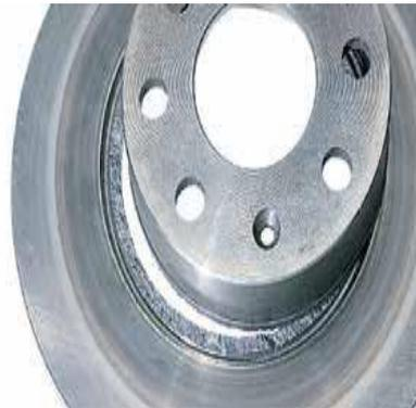
Figure 28: Usure non-uniforme(1-29)
