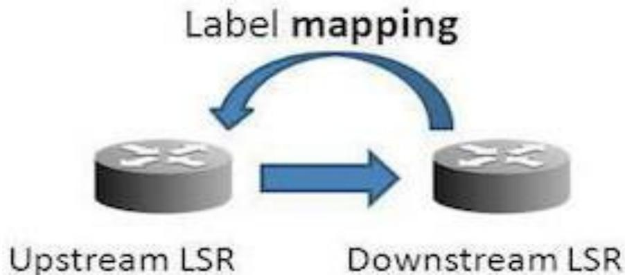
Figure II. 7. Principe du Downstream unsolicited [14]
