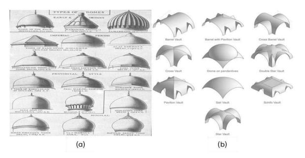
Figure 2-21 Sketches of domed and vaulted roof designs: (a)- domed roofs [194]; (b)vaulted roofs [195]
