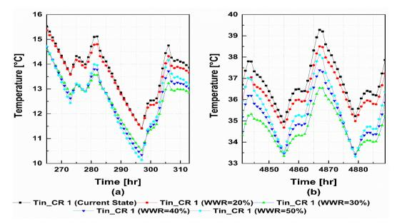
Figure 6-20 Comparison of internal temperature of classroom 1 in Winter (a) and Summer (b) for different Window-to-Wall Ratios (WWR)
