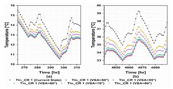
Figure 6-15 Effect of VSA on classroom 1's internal temperature: Winter (a) and Summer (b)
