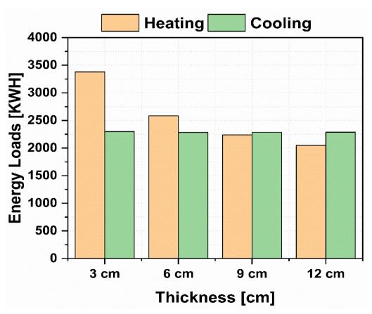
Figure 6-8 Heating and cooling requirements for the insulator wood fiber
