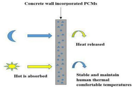
Figure 2-18 Functioning of concrete walls with incorporated Phase Change Materials (PCMs) for latent heat storage [170]
