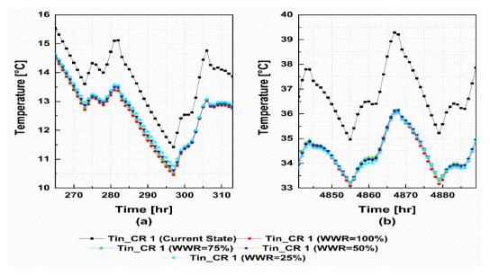
Figure 6-29 Indoor temperatures of classrooms 1: Impact of WWR on Winter (a) and Summer (b)
