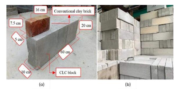
Figure 2-16 Comparison of Cellular Lightweight Concrete (CLC) blocks with conventional clay brick: (a)- Size comparison; (b)- Set of hardened CLC [165]
