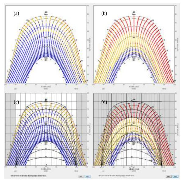
Figure 8-13 Sun shading chart;(a): Sun shading chart (Winter-Spring), (b): Sun shading chart (Summer-Fall), (c): Calculate the angle of shading (Horizontal and vertical shading), for Winter-Spring, (d): Calculate the angle of shading (Horizontal and vertical shading)
