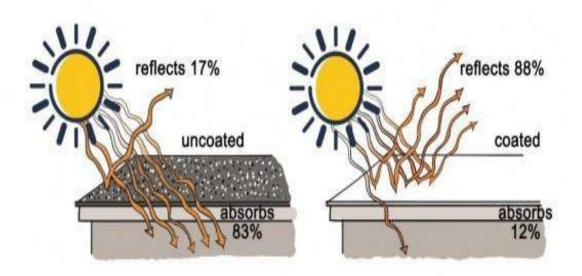
Figure 2-22 Comparison of uncoated and coated roofs for solar-reflective/cool roof applications [197]
