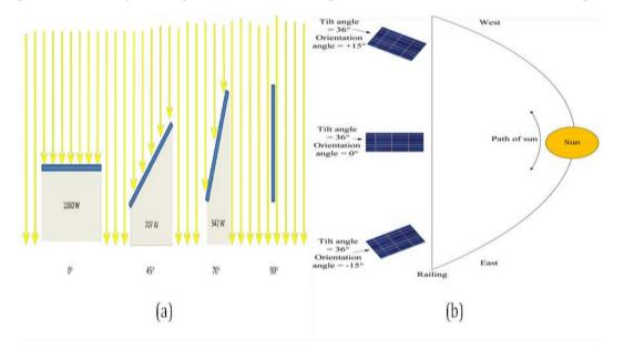
Figure 8-6 Solar radiation analysis; (a): Titled angle [347] and (b): Orientation angle [348]
