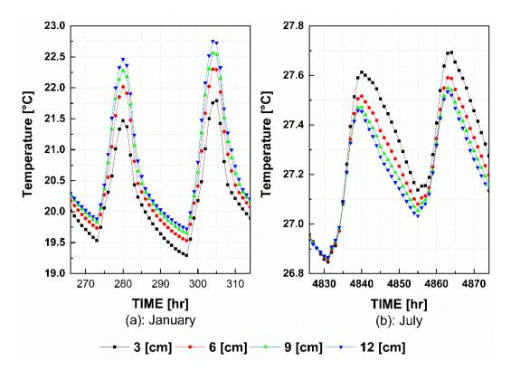
Figure 6-7 Distribution of the insulator wood fiber temperature where: (a) January; (b) July
