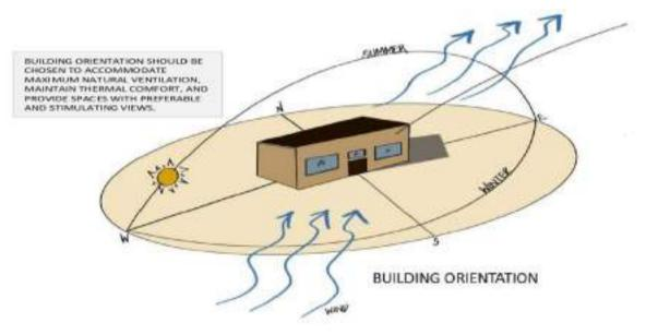
Figure 3-1 Building orientation and environmental analysis [224]
