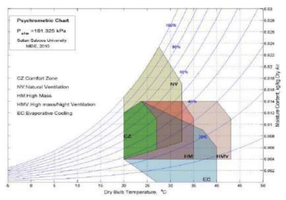
Figure 2-7 Givoni's bioclimatic chart [101]
