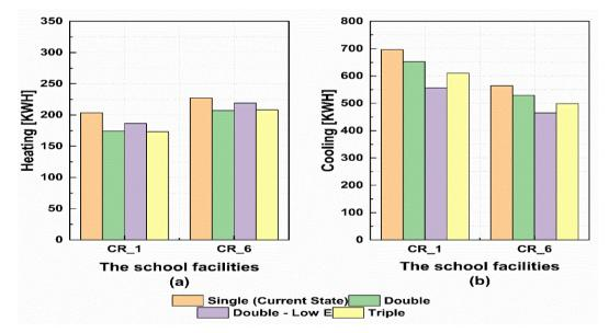
Figure 6-26 Energy loads comparison of classrooms 1 and 6 with different window glazing scenarios for Heating (a) and Cooling (b)
