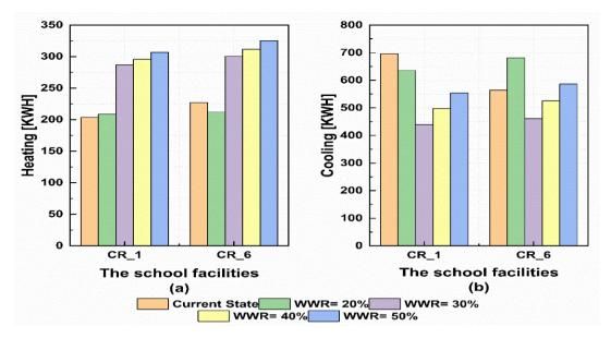
Figure 6-22 Energy loads of classrooms 1 and 6; (a): Heating, (b): Cooling
