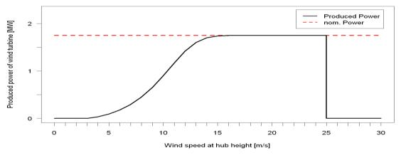
Figure 8-10 Power production of typical wind turbine [349]
