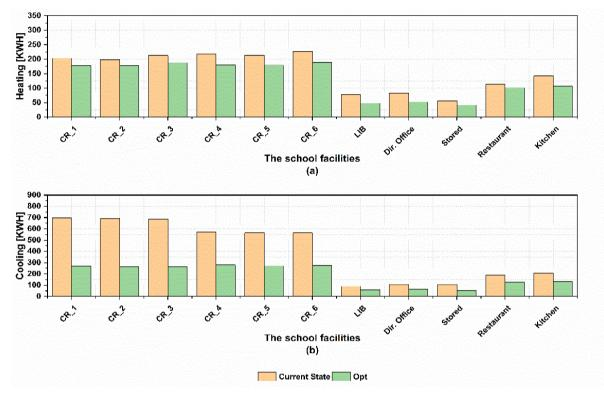
Figure 6-36 Annual heating and cooling needs for each facility: Comparison between the current state and optimized model with passive strategies
