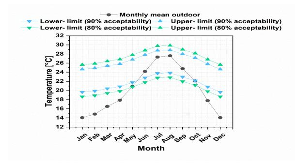
Figure 4-7 The monthly variation in the comfort temperature limits according to the ASHRAE 55-2010 standard
