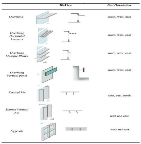
Figure 3-2 Types of shading devices and their optimum orientation [251]
