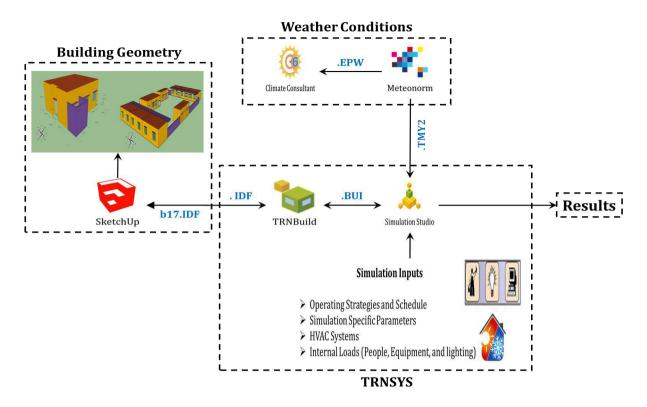
Figure 4-1 Diagrammatic representation of building performance simulation process
