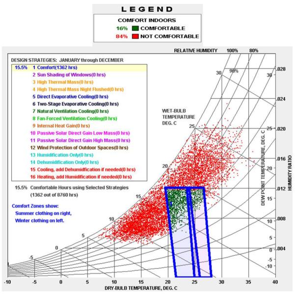
Figure 4-5 Psychrometric chart for village khoualed Abdel Hakem: Comfort Zone Figure 4-6 illustrates the optimal design solutions for constructing building envelopes in the village khoualed Abdel Hakem. The strategies have the capability to alter or screen extreme external climate conditions in order to establish pleasant inside settings in the village khoualed Abdel Hakem.
