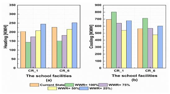
Figure 6-31 Impact of WWR on energy loads of classrooms 1 and 6 for heating and cooling
