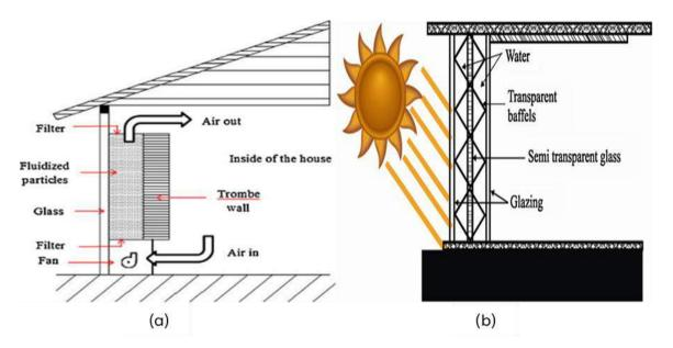
Figure 2-15 Passive solar walls: (a)- Visualization of fluidized Trombe wall system Components [160]; (b)- Transwall System: a cross-sectional perspective [162]
