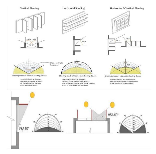
Figure 3-3 Schematic for calculating VSA, HAS [252]
