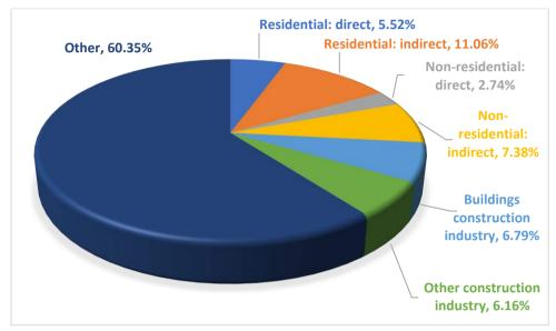
Figure 1-2 Global CO2 emissions from buildings, including embodied emissions from new construction, 2022 [5,6]
