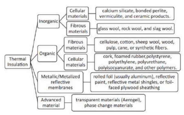
Figure 2-26 Various types of thermal insulation [112]
