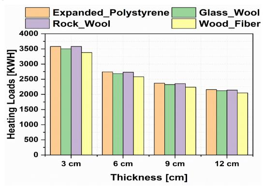
Figure 6-5 Heating loads for the insulators with various thicknesses Turning to Figure 6-6, we can see that wood fiber insulation also offers some savings in terms of cooling load reduction, with reductions of 1% to 2% across all thicknesses and compared to other insulation materials. While these savings may not be as significant as those associated with heating load reduction, they are still notable and can contribute to overall energy efficiency and cost savings in a building.
