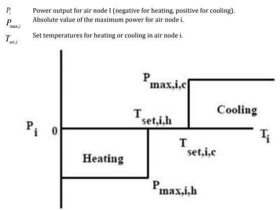
Figure 5-1 Power output versus temperature [310]
