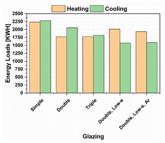
Figure 6-10 Heating and cooling demands of different glazing types
