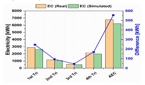
Figure 6-12 Comparison between the real and simulated energy consumption of the primary school
