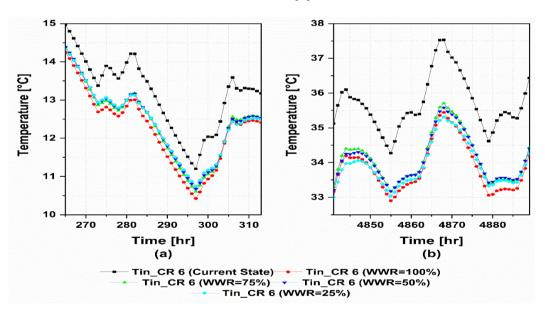
Figure 6-30 Indoor temperatures of classrooms 6: Impact of WWR on Winter (a) and Summer (b)
