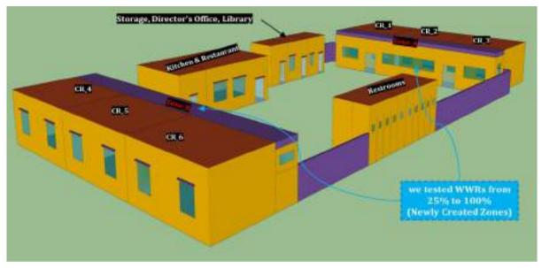
Figure 6-28 Building envelope adjustments showing newly added spaces on the Western and Eastern sides of the classrooms
