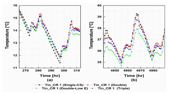
Figure 6-24 Comparison of internal temperature in classroom 1 with different types of glazing during Winter (a) and Summer (b)
