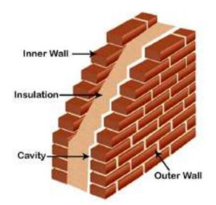
Figure 2-17 Schematic representation of ventilated or double-skin walls [166] Research by Barbosa and Ip [167] highlights the potential of double skin facades for naturally ventilated buildings, emphasizing their role in sustainable architecture. Tao et
