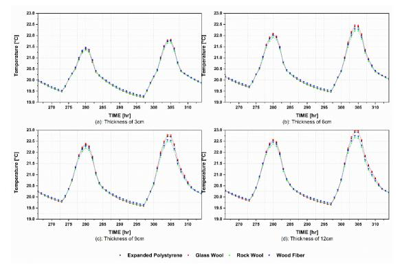
Figure 6-3 January temperatures with varying thicknesses of insulating materials where: (a) 3 cm; (b) 6 cm; (c) 9 cm; (d) 12 cm
