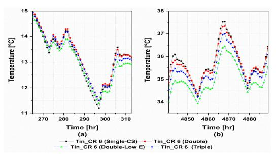
Figure 6-25 Comparison of internal temperature in classroom 6 with different types of glazing during Winter (a) and Summer (b)
