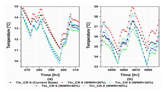
Figure 6-21 Comparison of internal temperature of classroom 6 in Winter (a) and Summer (b) for different Window-to-Wall Ratios (WWR)
