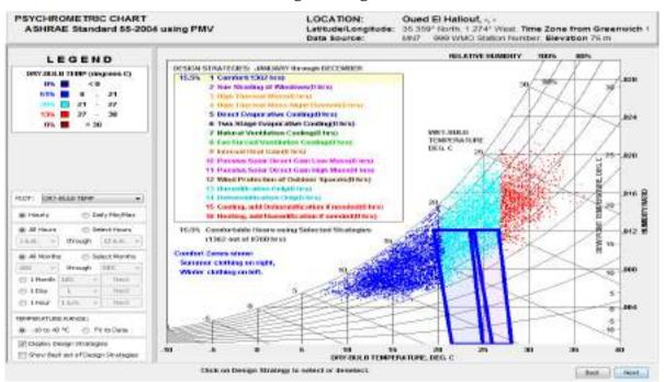
Figure 8-14 Psychrometric chart of dry bulb temperature, during all the year
