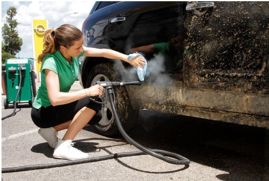
Figure 26 Car cleaning with a steam generator [25]
