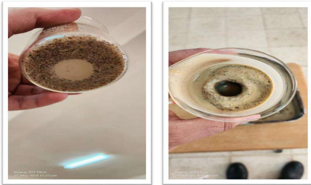
Figure 4.12 Results of Thixotropy on industrial bentonite (1minute)
