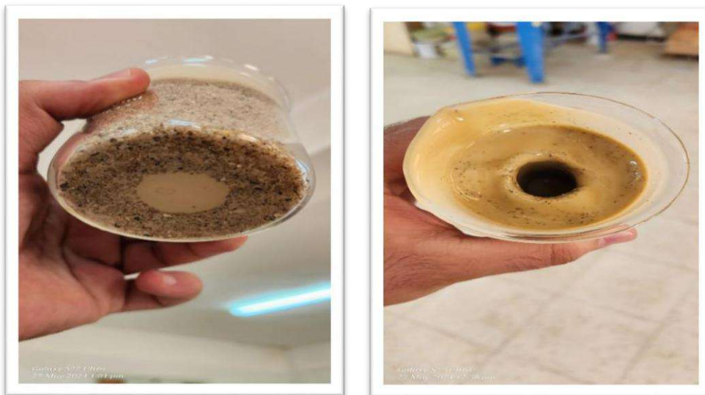
Figure 4.11 Results of Thixotropy on raw bentonite (2minute)
