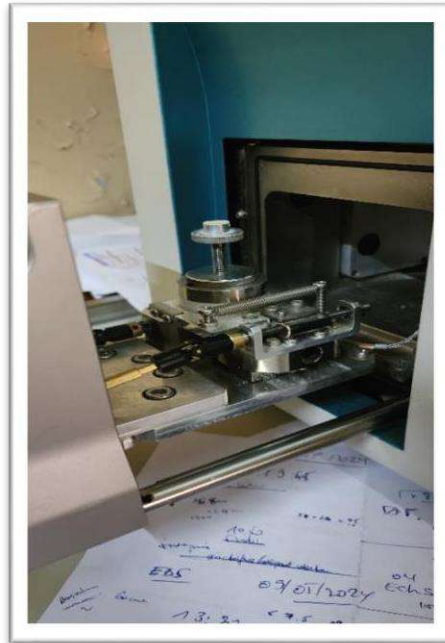
Figure 4.3 Placement of the sample in the microscope chamber
