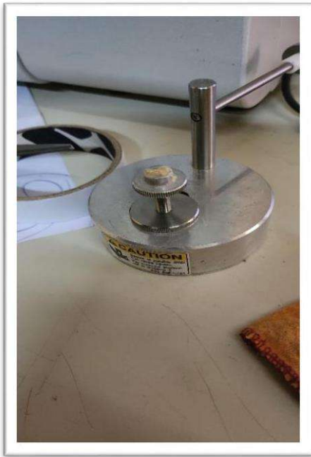
Figure 4.3 Placement of the sample in the microscope chamber
