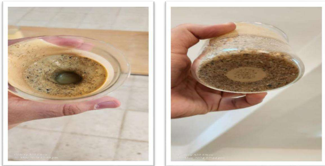
Figure 4.10 Results of Thixotropy on raw bentonite (1minute)
