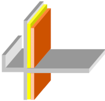
Figure 05 : linear thermal bridge [15]
