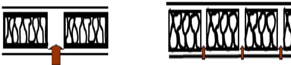
Figure 08 : Rule of thermal bridge division. [17]
