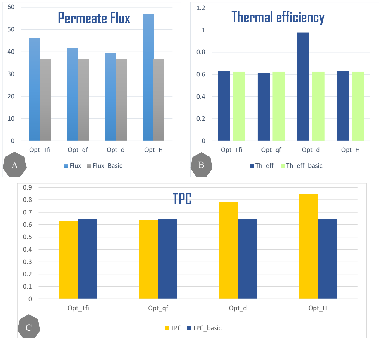
Figure III. 15: Obtained optimized parameters of the DCMD with its outputs.
