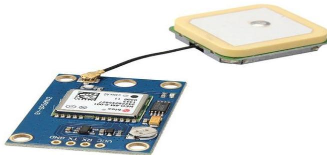
Figure 2.4: Module GPS (NEO-6) [6]
