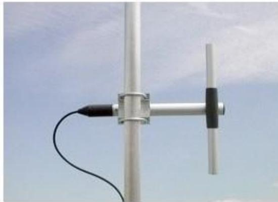
Figure I-10 : Antenne dipolaire [2]
