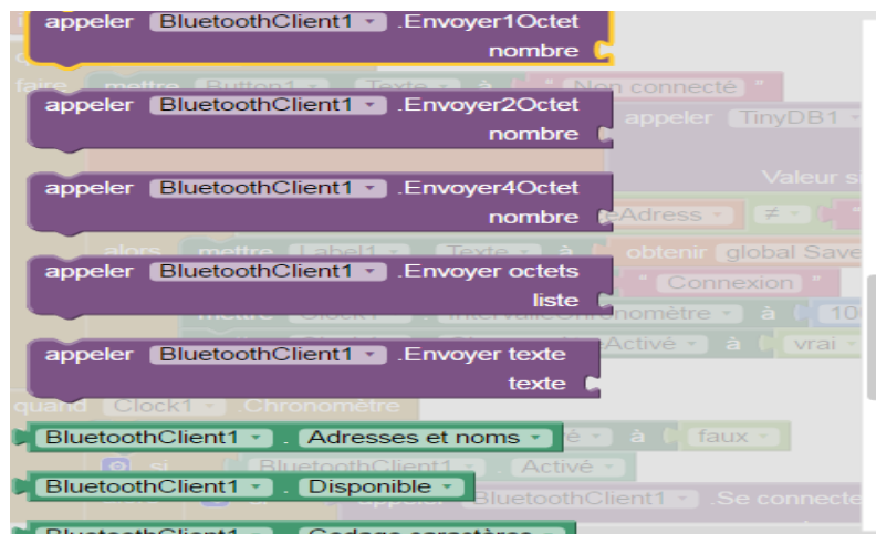
Fig.2.29. Blocs de Bluetooth Client.
