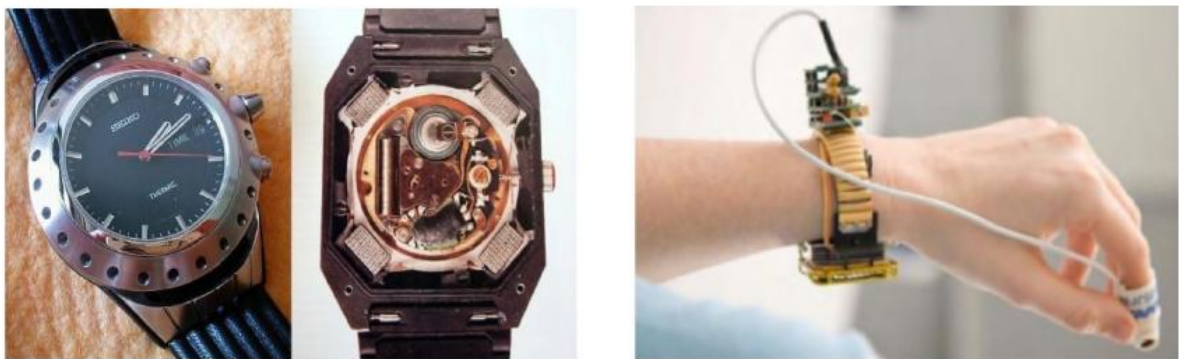
Figure.I.8: Watch and medical devices powered by thermoelectric devices [44]
