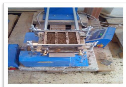
Figure 4.24: Appareil de chocs
