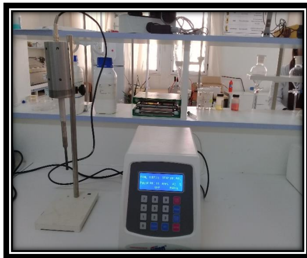
Figure 2: Appareil d'ultrason model OPTIC ivymen® SYSTEM CY-500.
