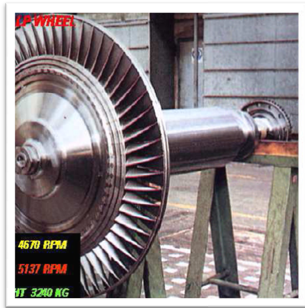
Fig.III.19 roue de turbine BP
