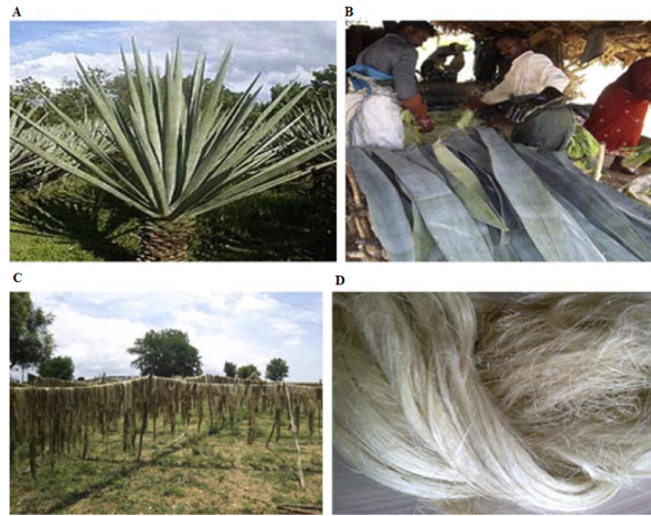
Figure 3.3: extraction of sisal fiber: (A)Sisal plant, (B) Decortication , (C) Drying, (D) Raw fiber [70].
