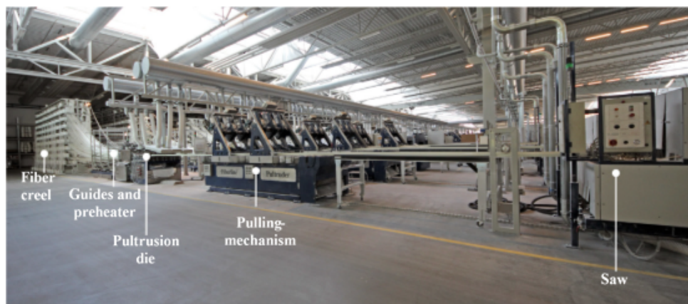
Figure 1.21: A state-of-the-art resin-injection pultrusion line [132].
