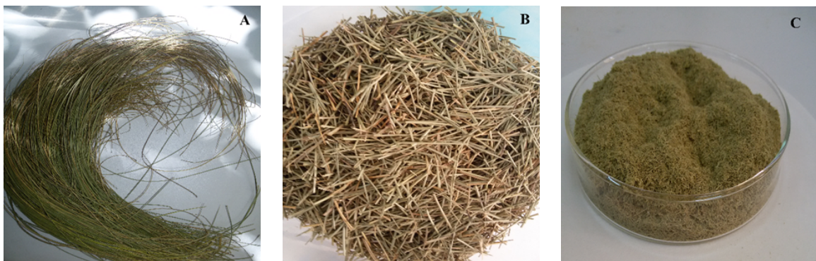
Figure 2.4: Physical preparation of the Alfa fibres, (A) The Alfa stems gathered. (B) The Cut Alfa stems. (C) The Alfa fibres collected from a 250 \mu m diameter sieve.
