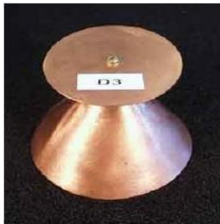
**Figure II. 10:** Antenne discône [35]
