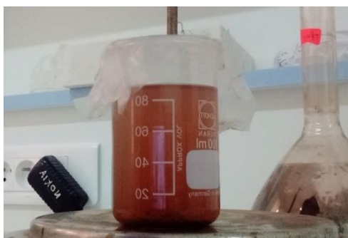
Figure-II; 10; a setup of solution containing support, ultrapure water, silver nitrate and plant leaf extract that has been left for 3days with continuous stirring
