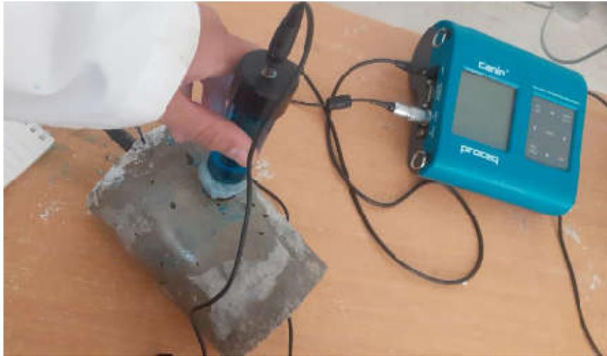
FIGURE 2. 5 APPAREIL DE MESURE POTENTIEL (CANIN+) (PRISE PAR LES AUTEURS)
