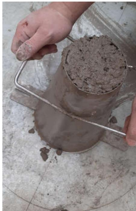
FIGURE3. 12 ESSAI D'AFFAISSEMENT DE CONE D'ABRAMES
