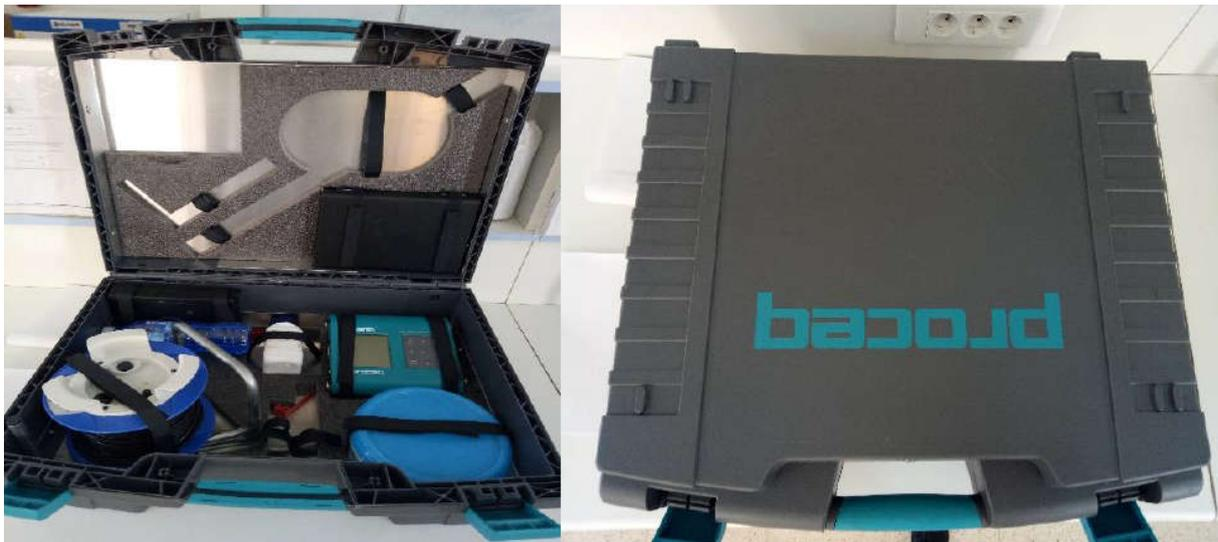
FIGURE 2. 16 APPAREIL DE MESURE POTENTIEL CANIN+ PRISE PAR LES AUTEURS
