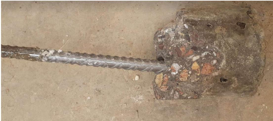
FIGURE3. 19 : PRESENT PHOTO DE L' ARMATURE APRES LA DESTRUCTION
