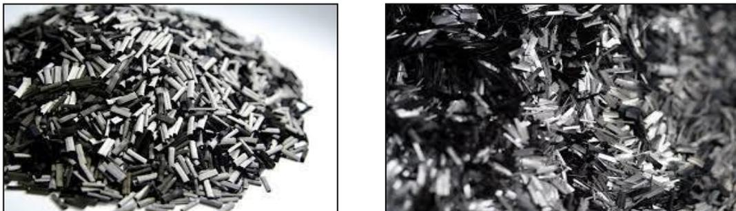
Figure 1.4: Fibres de carbone.
