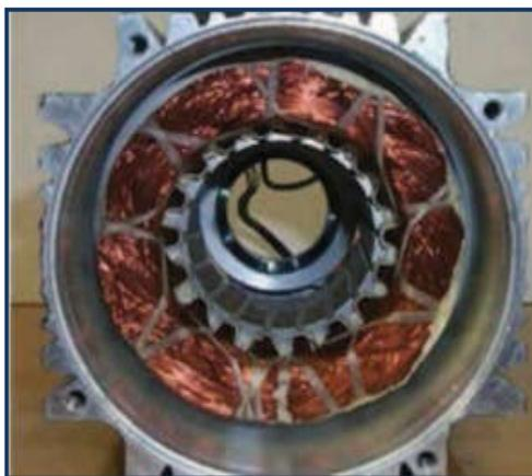
**Figure I.2** Stator de l'MSAP
