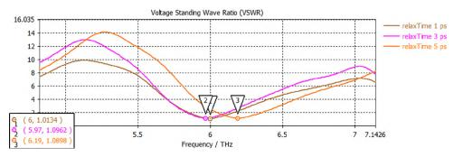
FIG. 4: VSWR of proposed antenna with different relax time 1 ps, 3 ps, and 5 ps
