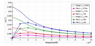
FIGURE 3. Graphene conductivity curve variation with respect to chemical potential ( $\mu c$ ) for  $\tau = 0.1$  ps at T = 300 K [1].
