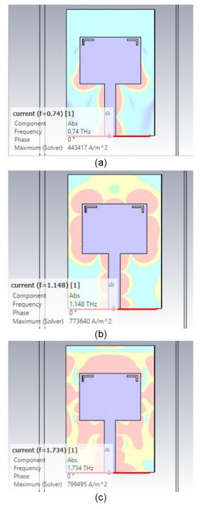
**FIG. 7:** Current density: (a) in frequency 0.74 THZ; (b) in frequency 1.148 THZ; and (c) in frequency 1.734 THZ
