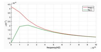
FIGURE 2. Graphene conductivity curve with properties  $\mu c = 0 \text{ eV}$ and  $\tau = 0.1 \text{ ps at } T = 300 \text{ K}$  [1].
