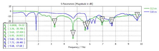
FIG. 3: S11 parameter with chemical potential values of 0.2 and 0.8 eV
