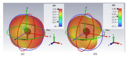
**FIG. 8:** (a) 3D radiation pattern of the antenna at 1.8 eV for f = 5.53 THz; and (b) 3D radiation pattern of the antenna for f = 7.24 THz
