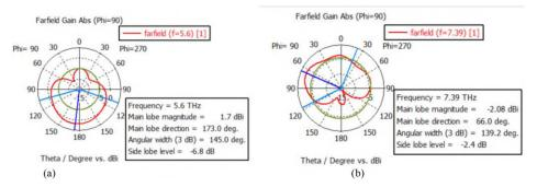
**FIG. 14:** (a) Polar radiation pattern of the antenna at 0.2 eV for f = 5.6 THz; and (b) polar radiation pattern of the antenna at 0.2 eV for f = 7.39 THz
