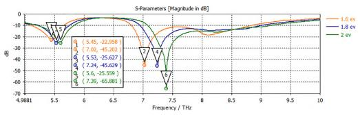
FIG. 4: S11 parameter with chemical potential values of 1.6, 1.8, and 2 eV
