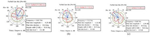
**FIG. 11:** (a) Polar radiation pattern of the antenna at 0.8 eV for f = 5.82 THz; (b) polar radiation pattern of the antenna at 0.8 eV for f = 7.72 THz; and (c) polar radiation pattern of the antenna at 0.8 eV for f = 9.68 THz
