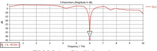
FIG. 2: Reflection coefficient S11 of proposed antenna
