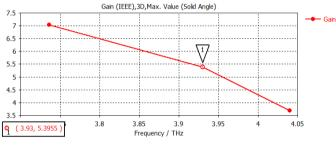
Fig. 5. Gain of proposed antenna with Silicon substrate
