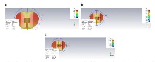
**FIG. 6:** 3D radiation pattern of proposed antenna with different relax time (a) 1 ps; (b) 3 ps; and (c) 5 ps
