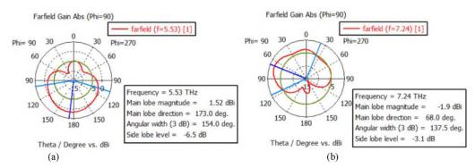
**FIG. 13:** (a) Polar radiation pattern of the antenna at 1.8 eV for f = 5.53 THz; and (b) polar radiation pattern of the antenna for f = 7.24 THz
