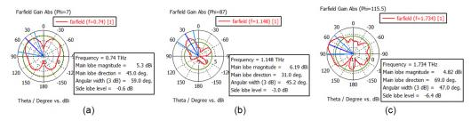
**FIG. 5:** Polar radiation pattern: (a) in frequency 0.74 THZ; (b) in frequency 1.148 THZ; and (c) in frequency 1.734 THZ
