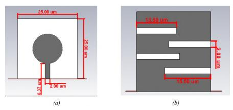
**FIG. 1:** (a) Front view of the circular proposed graphene patch antenna; (b) rear view of the circular proposed graphene patch antenna
