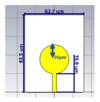
Fig. 2. Proposed nano circular patch antenna
