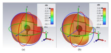
**FIG. 7:** (a) 3D radiation pattern of the antenna at 1.6 eV for f = 7.02 THz; and (b) 3D radiation pattern of the antenna at 1.6 eV for f = 5.4 THz
