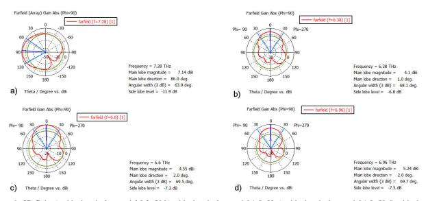
FIGURE 9. 3D Gain a) with chemical potential 0.2 eV, b) with chemical potential 1.5 eV, c) with chemical potential 1.8 eV, d) with chemical potential 2 eV.
