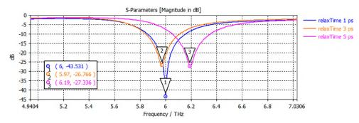
FIG. 3: Reflection coefficient S11 of proposed antenna with different relax time 1 ps, 3 ps, and 5ps
