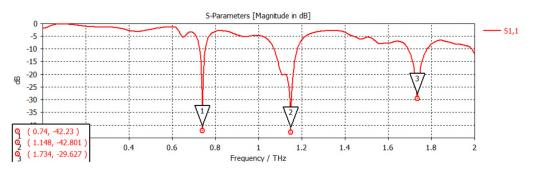
FIG. 2: Reflection coefficient S11 of proposed antenna
