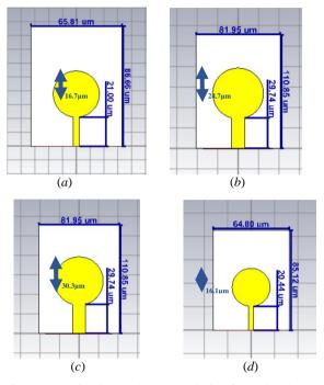
Fig. 7. Nano circular patch antenna design for each substrate: (a) Alumina, (b) RogersRO4003C, (c) RT Duriod 5850, and (d) RT Duriod 3210
