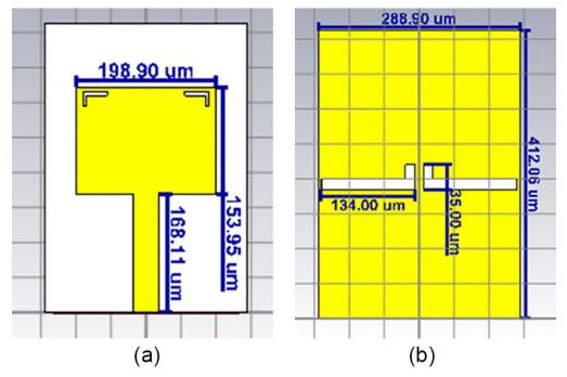
**FIG. 1:** (a) Front view of the rectangular proposed patch antenna; (b) rear view of the rectangular proposed patch antenna
