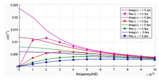
FIGURE 4. Graphene conductivity curve variation with respect to relaxation time ( $\tau$ ) for  $\mu c = 0$  eV at T = 300 K [1].
