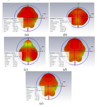
Fig. 12. 3D radiation pattern of the antenna: (a) Alumina substrate,
