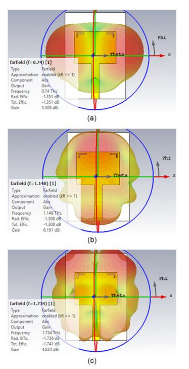
**FIG. 6:** 3D radiation pattern: (a) in frequency 0.74 THZ; (b) in frequency 1.148 THZ; and (c) in frequency 1.734 THZ
