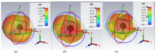
**FIG. 6:** (a) 3D radiation pattern of the antenna at 0.8 eV for f = 5.82 THz; (b) 3D radiation pattern of the antenna at 0.8 eV for f = 7.72 THz; and (c) 3D radiation pattern of the antenna at 0.8 eV for f = 9.68 THz
