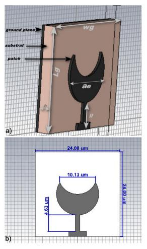
FIGURE 1. The Crescent Proposed Graphene patch antenna, a) antenna design, b) antenna dimensions.
