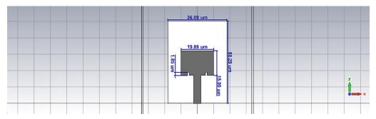
FIG. 1: The rectangular proposed graphene patch antenna
