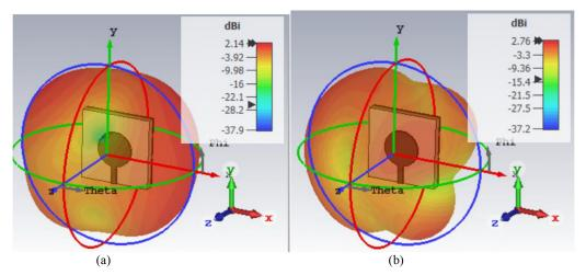
**FIG. 9:** (a) 3D radiation pattern of the antenna at 0.2 eV for f = 5.6 THz; and (b) 3D radiation pattern of the antenna at 0.2 eV for f = 7.39 THz
