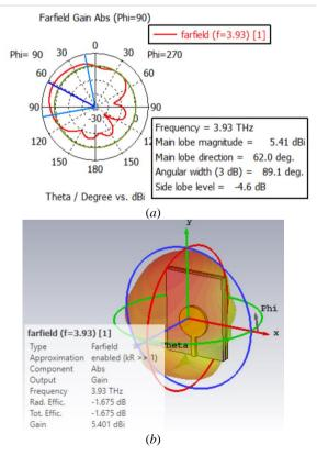
Fig. 6. Radiation pattern of the proposed antenna: (a) polar radiation pattern, and (b) 3D radiation pattern
