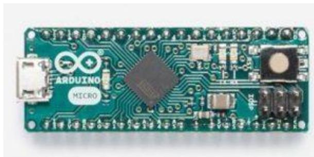
**Figure 5:** Arduino Micro
