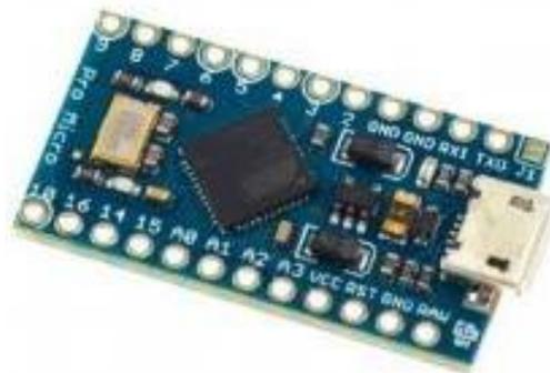
Figure 14: Micro Arduino Pro
