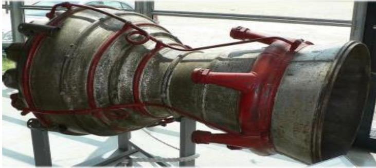
Figure III-2: La tuyère de V-2. [14]
